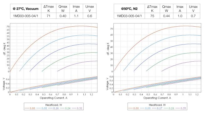
**Note**: Performance data is specified for optimal conditions (TEC hot side is stabilized at ambient temperature). Heatsink thermal resistance is not included into estimations. Use TECCad Software for estimations under different conditions.
